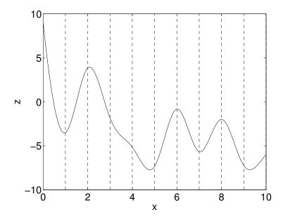
In approximation problems with splines it is convenient to parametrize a spline as a linear combination of basis functions, called *B-splines*. The precise definition of B-splines is not important for our purposes; it is sufficient to know that every cubic spline can be written as a linear combination of M+3 cubic B-splines  $g_k(t)$ , *i.e.*, in the form
